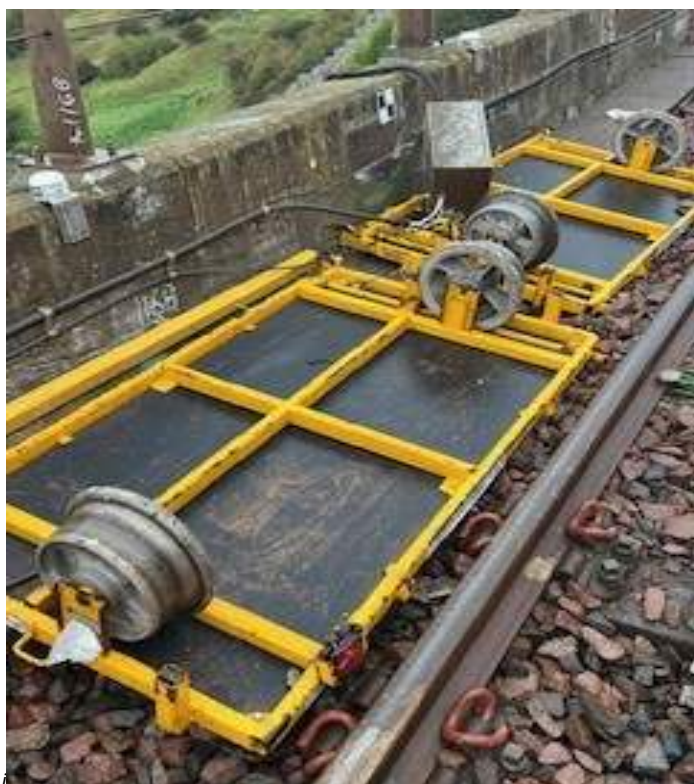
Track Trolleys located in the cess above and the damage caused
